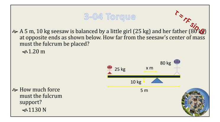
$\sum \tau = 0$   $(2.5 m + x)(25 kg \cdot 9.8 m/s^2) + x(10 kg \cdot 9.8 m/s^2) - (2.5 m - x)(80 kg \cdot 9.8 m/s^2)$  = 0 612.5 Nm + 245 N x + 98 N x - 1960 Nm + 784 N x = 0 -1347.5 Nm + 1127 N x = 0 1127 N x = 1347.5 Nm x = 1.20 m  $\sum F = -W_g - W_f - W_b + F_f = 0$   $-(25 kg) \left(9.8 \frac{m}{s^2}\right) - (80 kg) \left(9.8 \frac{m}{s^2}\right) - (10 kg) \left(9.8 \frac{m}{s^2}\right) + F_f = 0$   $-1127 N + F_f = 0$   $F_f = 1127 N$
