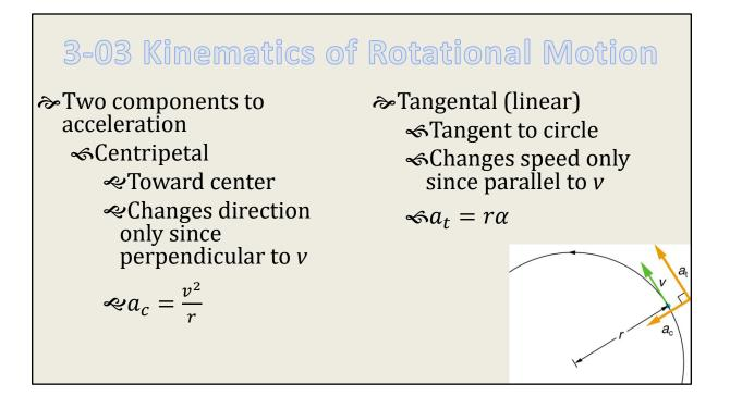
Equations of kinematics for rotational motion are same as for linear motion
